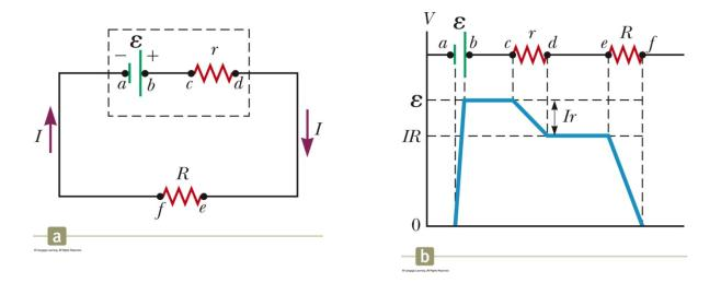
r = internal resistance of battery  $\boxed{V_{ad} = IR} \text{ EMF voltage}$   $\boxed{V_{ad} = \varepsilon - Ir} \text{ Terminal voltage is NOT equal to the EMF voltage}$   $IR = \varepsilon - Ir$   $IR + Ir = \varepsilon$   $\boxed{I = \frac{\varepsilon}{R+r}} \text{ Current with a real battery}}$   $\boxed{I\varepsilon = I^2R + I^2r} \text{Power delivered to internal resistance}}$ Power delivered by battery
