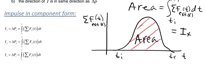
In a F(t) vs. t graph the area between the curve and the time axis equals the impulse during the corresponding time interval.
