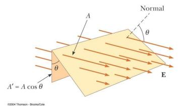
Since the same number of electric field lines cross both surfaces, the flux must be the same through both surfaces. The surface areas are related by:
