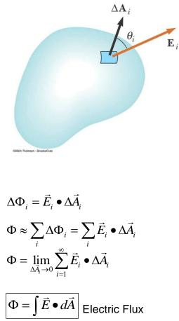
Recall that electric flux is proportional to the number of electric field lines crossing a surface. For a closed surface, electric field lines will be either entering or leaving the surface and thus the corresponding flux may be positive or negative.
