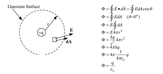
Note that this result is independent of *r* and thus holds true for any spherical surface. This result holds true for any closed surface surrounding the charge because the flux must be the same.
