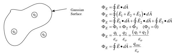
\*  $\vec{E}$  = total electric field at any point on the Gaussian surface due to all surrounding charges.
