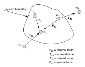
A diagram of the external forces acting on a system is called a Free-Body Diagram.
